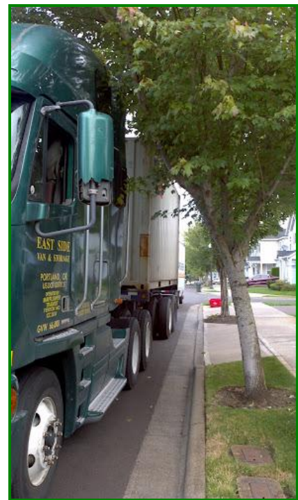
Branches over the road require this truck to park far from the curb. Clearance of 14' is recommended.
